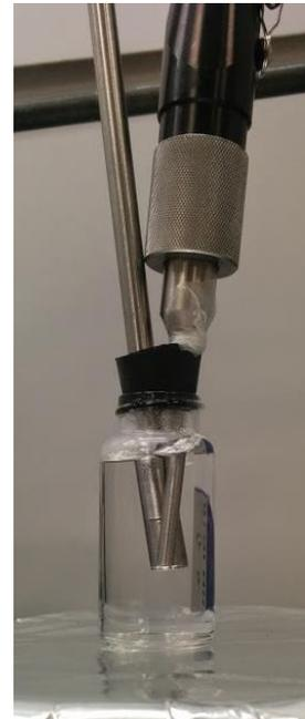
**Figure 1. Compact sample interface: IR and Raman probes in a 20 mL vial filled with water.**
