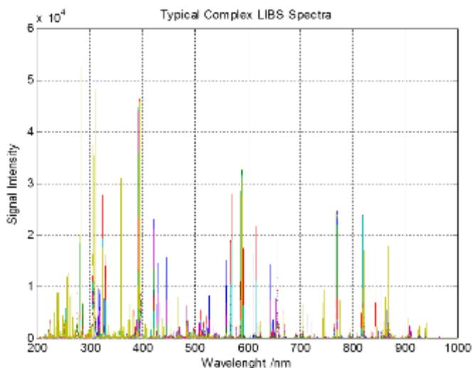
Figure 2 - Typical complex LIBS spectra
