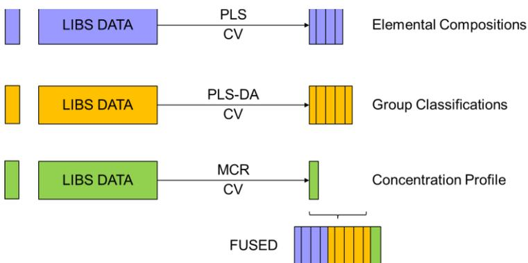
Figure 3 - High level data fusion schematic
