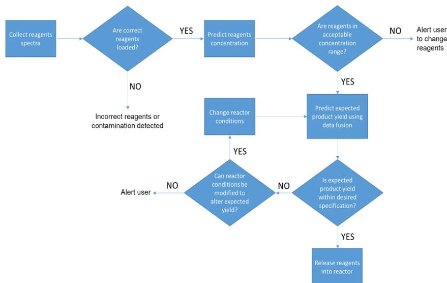
Figure 1 - Basic Outline of Feed-forward model architecture
